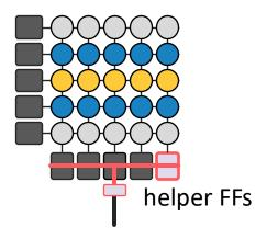
Helper flip-flops latches and drives source column into the destination column
