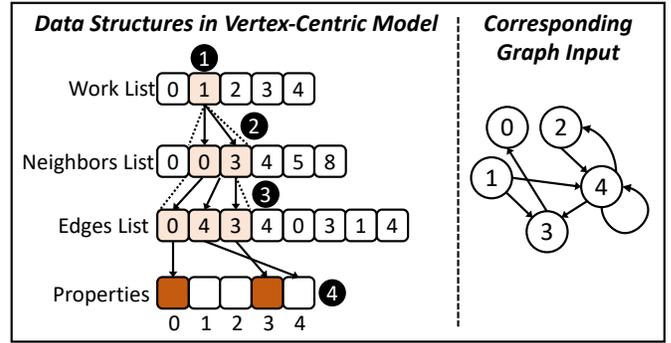
**Figure 3: Data-dependent accesses in vertex-centric graph processing model.**
