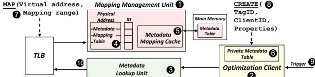
Figure 1: MetaSys hardware components and operation. MetaSys’ structures are highlighted.
