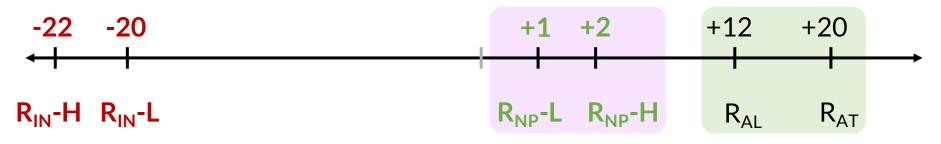
AT = Accurate & timely; AL = Accurate & late; NP = No-prefetching; IN = Inaccurate; H = High mem. b/w; L = Low mem. b/w
