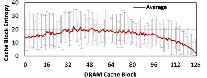
Figure 10: Average entropy of each cache block in the highest-entropy segment in all modules. The error bars show the range of the values across all modules.
