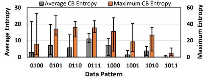
Figure 8: Average (grey bars, left Y-axis) and maximum (orange bars, right Y-axis) DRAM cache block entropies for different data patterns across 17 modules. The error bars show the range of the average and the maximum DRAM cache block entropy across all modules.
