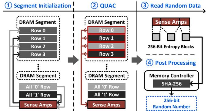
Figure 6: QUAC-TRNG mechanism.
