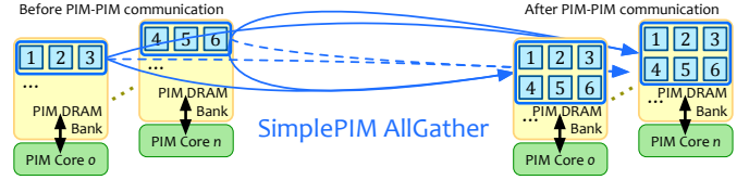
Figure 5: SimplePIM AllGather function (example with two PIM cores)
