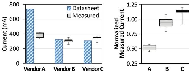
Figure 9: IDD4R current measurements (left), and current normalized to datasheet value (right).
