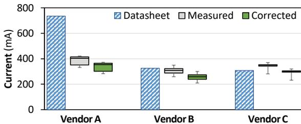
Figure 10: IDD4R current measurements before and after correction for I/O driver current.
