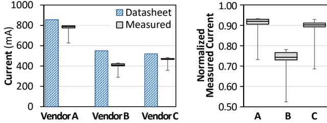
Figure 13: IDD5B current measurements (left), and current normalized to datasheet value (right).
