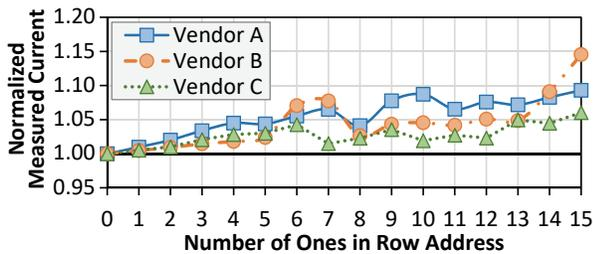
**Figure 22: Relationship between activation current and number of ones in row address, normalized to activation current for Row 0.**
