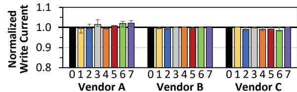
Figure 21: Write current variation across banks, normalized to current for Bank 0. Error bars indicate the 25th and 75th percentile measurements.
