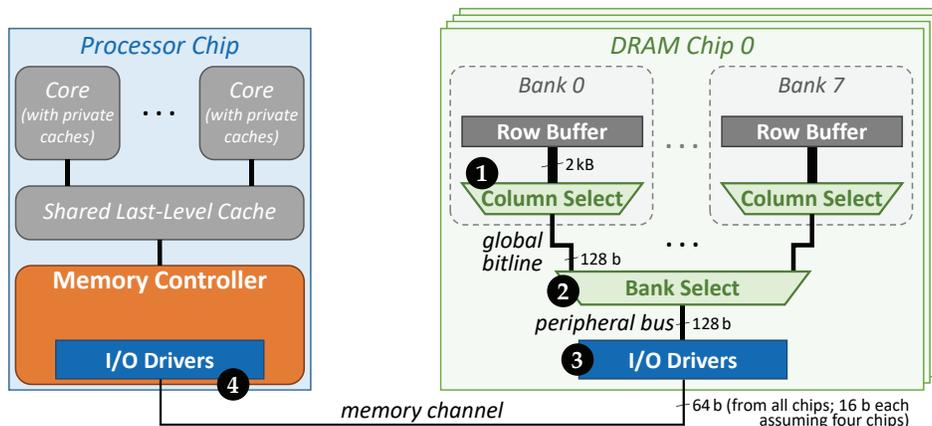
Figure 3: Overview of peripheral circuitry and I/O in a four-chip DRAM module.
