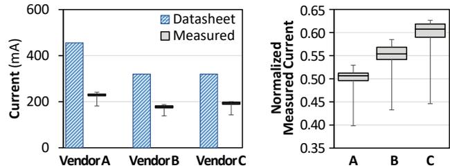
Figure 11: IDD4W current measurements (left), and current normalized to datasheet value (right).
