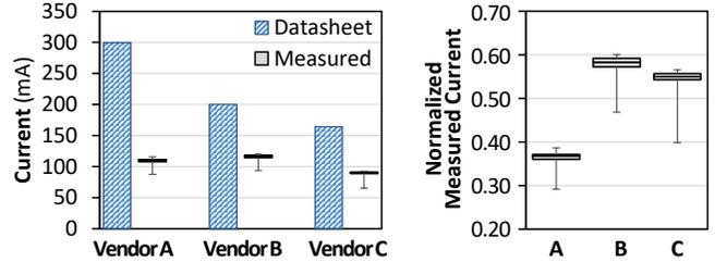
Figure 8: IDD1 current measurements (left), and current normalized to datasheet value (right).
