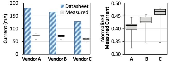
Figure 7: IDD0 current measurements (left), and current normalized to datasheet value (right).
