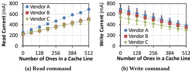
**Figure 15: Effect of the number of ones on the read (left) and write (right) current drawn by DRAM. Error bars indicate the 25th and 75th percentile measurements.**
