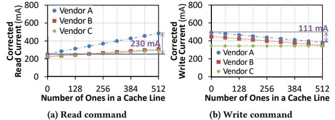
**Figure 16: Effect of the number of ones on the read (left) and write (right) current drawn by DRAM, after subtracting a conservative estimate of the I/O driver current.**
