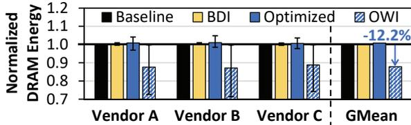
**Figure 26: Average energy consumption for various cache-line-level data encodings, normalized to energy consumed with *Baseline* encoding. Error bars show maximum and minimum normalized energy values across all applications.**
