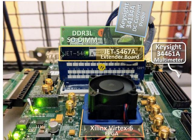
Figure 4: Our experimental infrastructure connected to an FPGA to measure DRAM current.
