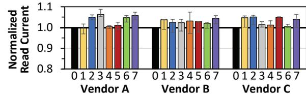
Figure 20: Read current variation across banks, normalized to current for Bank 0. Error bars indicate the 25th and 75th percentile measurements.
