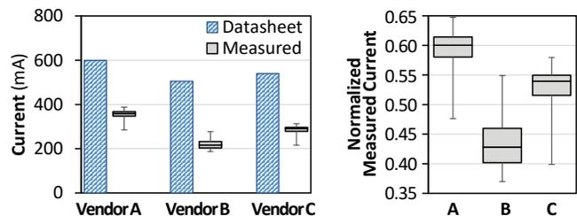
Figure 12: IDD7 current measurements (left), and current normalized to datasheet value (right).
