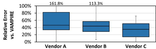
Figure 25: Box plots showing the distribution of the relative error for the DRAMPower model compared to VAMPIRE, across the applications that we simulate. Each box illustrates the quartiles of the distribution of the relative error for each application, and the whiskers illustrate the minimum and maximum error values, across all applications evaluated.
