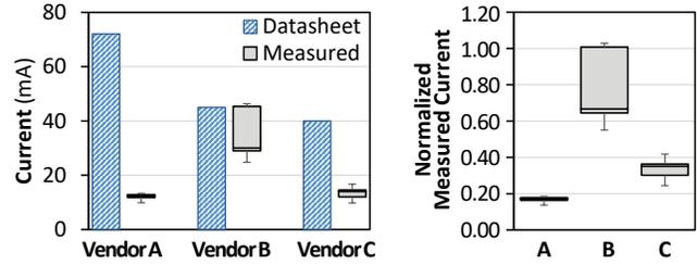
Figure 14: IDD2P1 current measurements (left), and current normalized to datasheet value (right).
