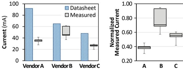
Figure 5: IDD2N current measurements (left), and current normalized to datasheet value (right).
