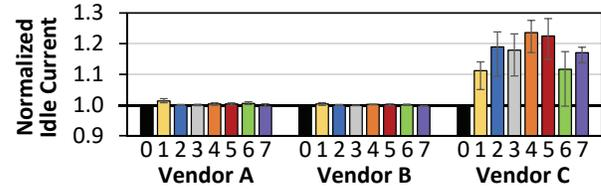
Figure 19: Idle current variation across banks when one bank is active, normalized to current for Bank 0. Error bars indicate the 25th and 75th percentile measurements.
