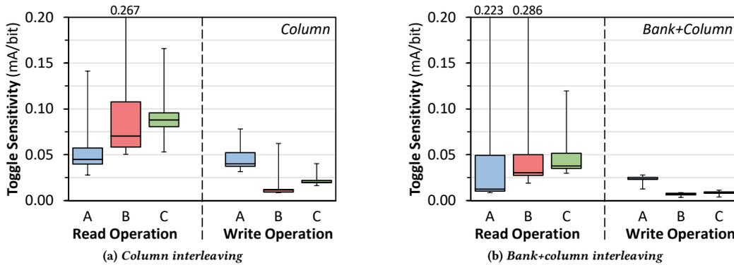
Figure 18: Effect of bit toggling on read and write current consumption.
