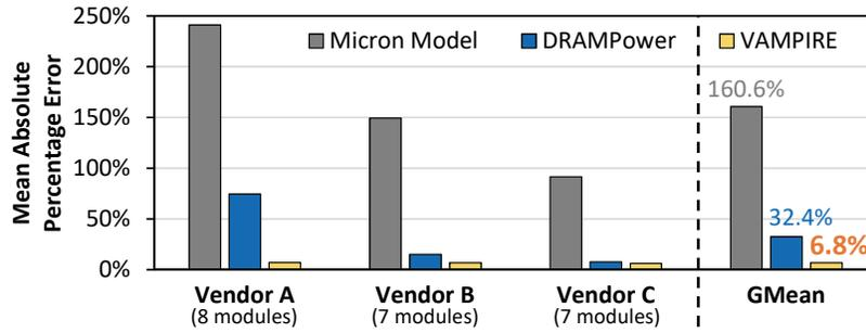
Figure 24: Mean absolute percentage error of state-of-the-art DRAM power models and of VAMPIRE, compared to real measured DRAM power.
