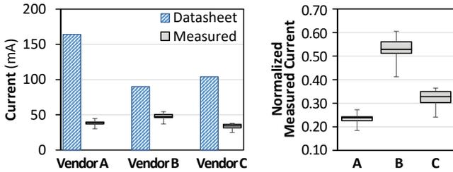
Figure 6: IDD3N current measurements (left), and current normalized to datasheet value (right).
