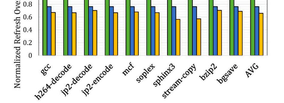
On average, refresh performance overhead reduces by 23% using VRL and 34% using VRL-Access
