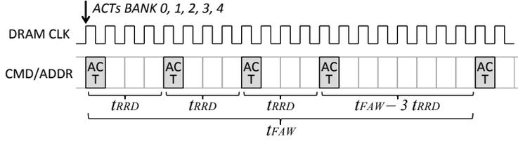
Figure 2: Inter-bank row-activate timing constraints
