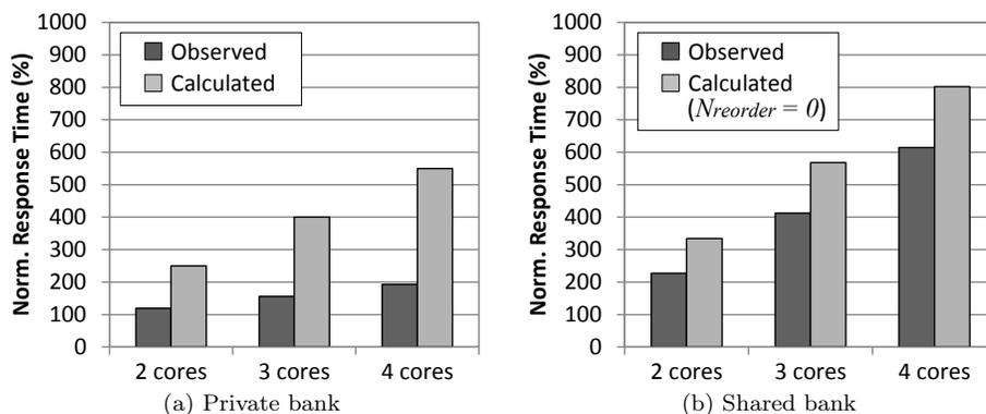
Figure 7: Response times of a synthetic task that generates multiple outstanding read and write memory requests at a time
