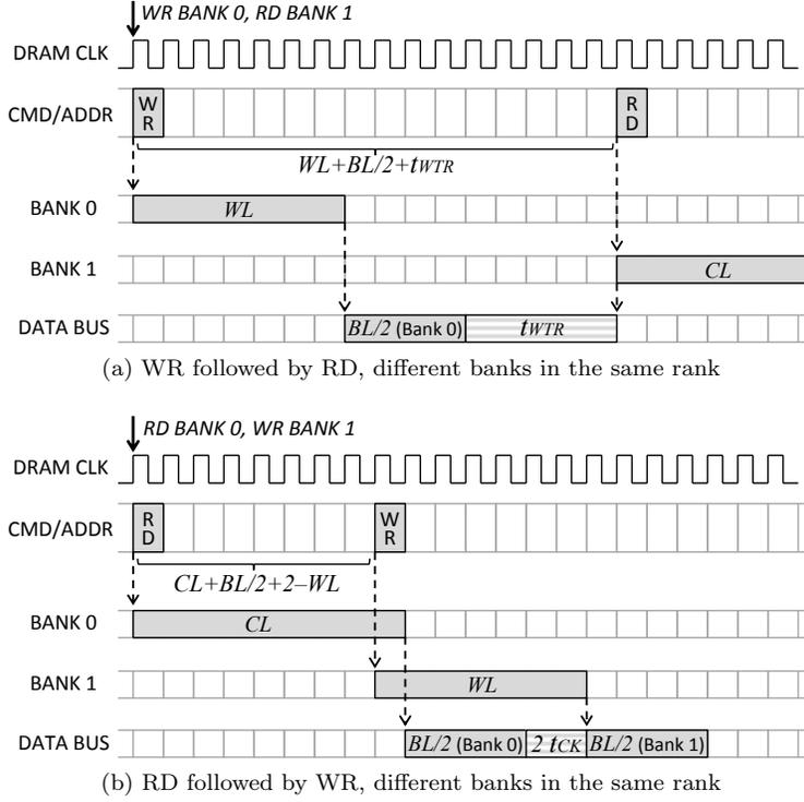
Figure 3: Data bus turn-around delay
