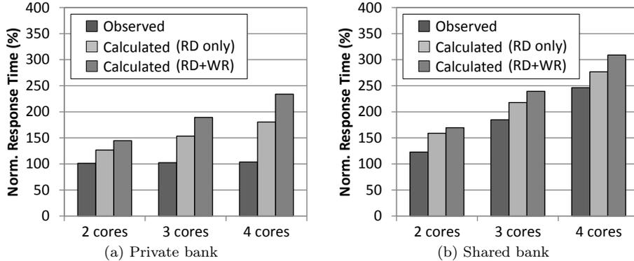
Figure 6: Response times of a synthetic task that generates one outstanding read memory request at a time
