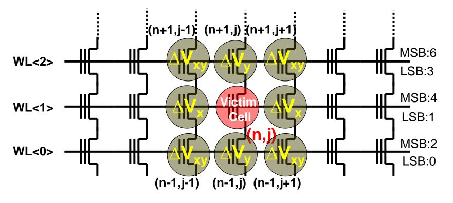
What affects cell-to-cell program interference in Flash chips? How to accurately model cell-to-cell program interference?
