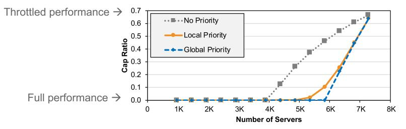
Using 1% cap ratio as threshold, our system supports 5832 servers, while Local Priority only supports 4860 servers
