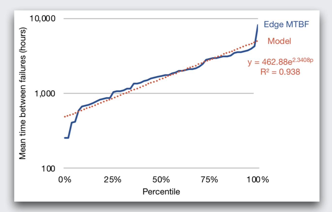
Typical edge node failure rate is on the order of months
