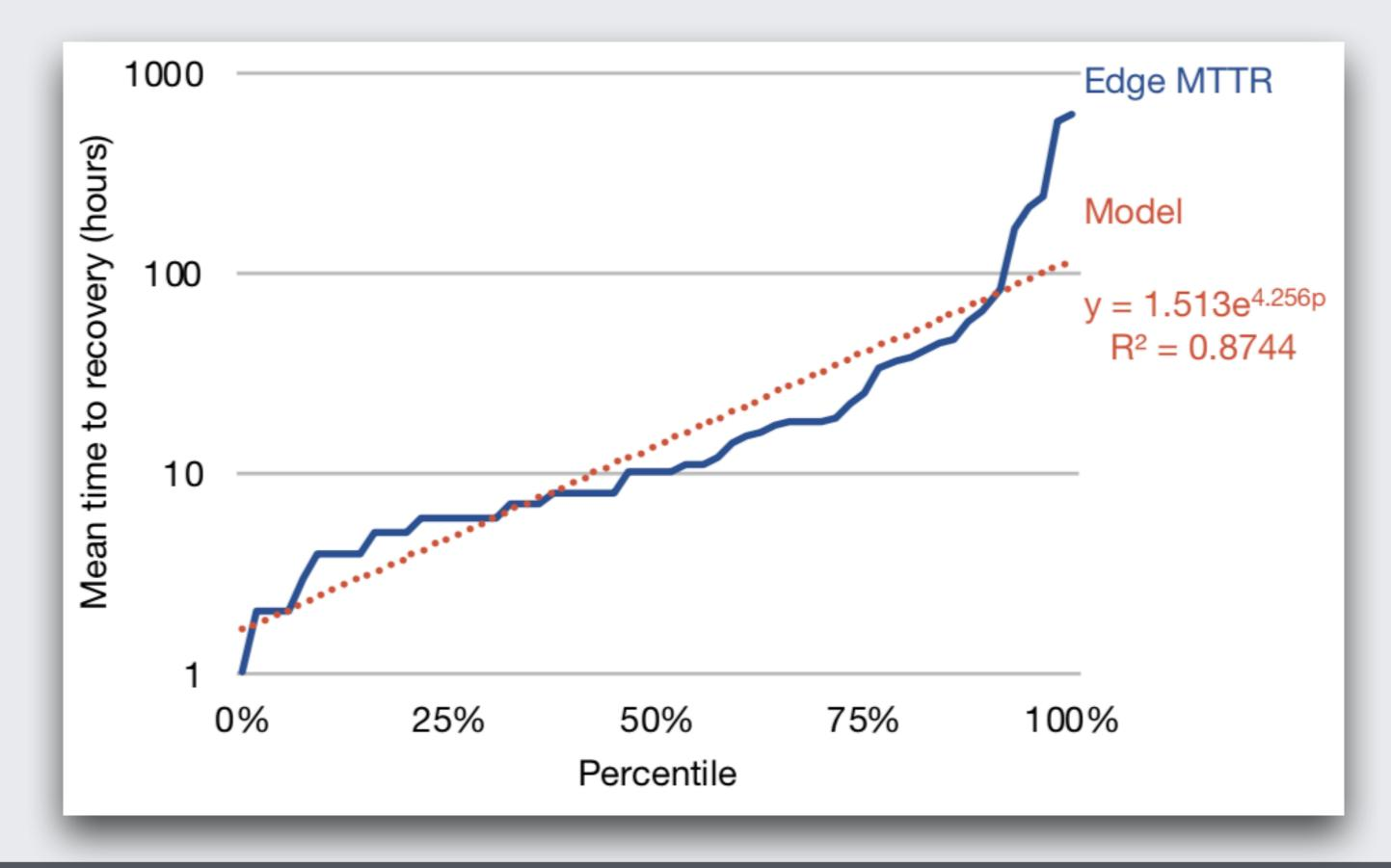
Edge node mean time to repair is on the order of hours
