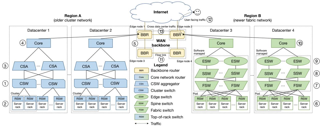
**Figure 1: Facebook’s network architecture, explained in §3. Data centers use either an older cluster network or a newer fabric network. Cluster networks and fabric networks communicate through the WAN backbone and Internet.**
