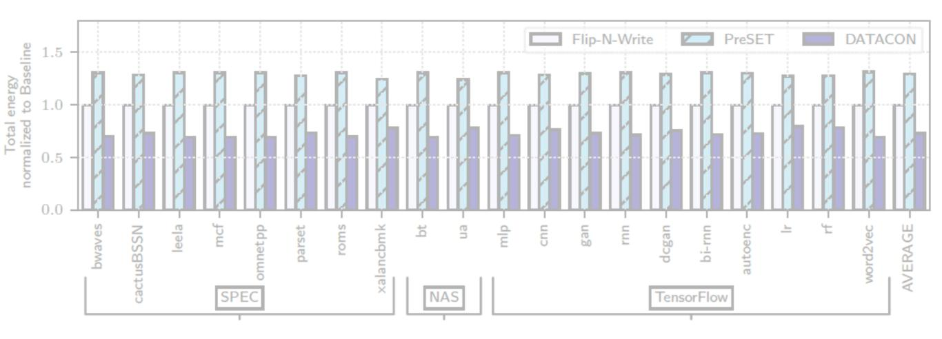
Average Energy of DATACON is 27% lower than Baseline, 26% lower than Flip-N-Write, and 43% lower than PreSET
