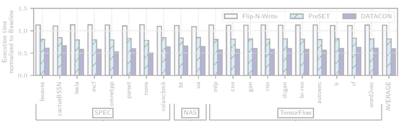
Average Execution time of DATACON is 40% lower than Baseline, 47% lower than Flip-N-Write, and 27% lower than PreSET
