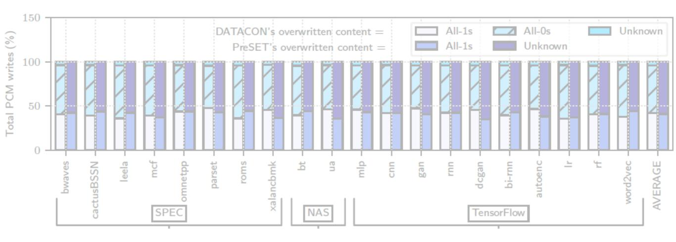
DATACON overwrites unknown content for only 4% of PCM writes. PreSET overwrites unknown content for 59% of PCM writes.
