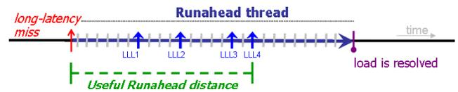
Figure 2: Illustration of the “useful runahead distance” under a runahead thread execution
