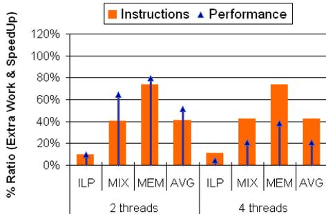
Figure 1: Extra executed instructions vs. performance SpeedUp due to Runahead Threads.
