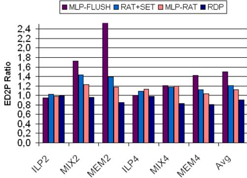
Figure 8: Energy-Delay<sup>2</sup> of evaluated Runahead thread techniques
