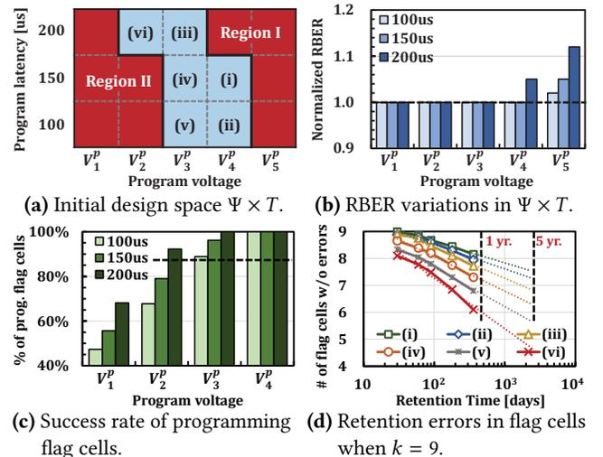
**Figure 9.** Design space exploration results for pLock.
