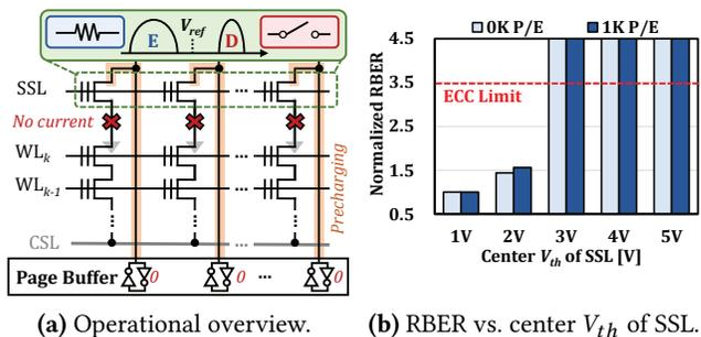
(a) Operational overview. (b) RBER vs. center  $V_{th}$  of SSL.
