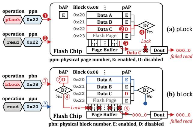
Figure 7. Operational overview of pLock and bLock.
