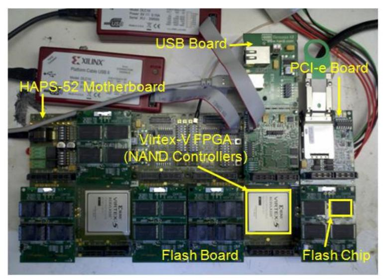
FPGA-based flash memory testing platform [Cai+,FCCM '11]
