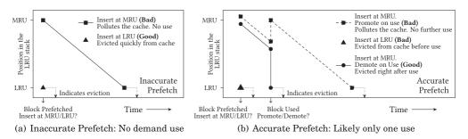
Fig. 2. Effect of different policies on the cache occupancy of (a) an inaccurate and (b) an accurate prefetch. Each line corresponds to a specific insertion/promotion policy followed for prefetched blocks.
