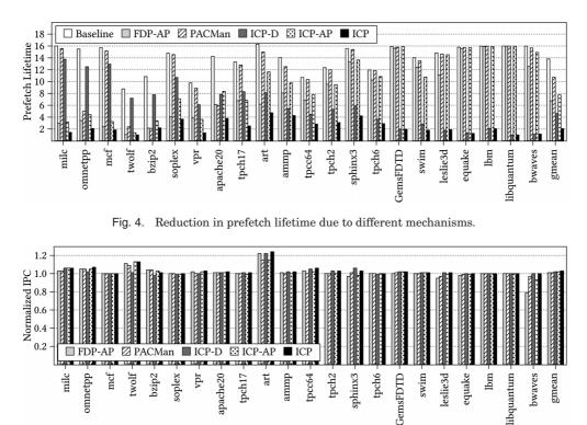
Fig. 5. Effect of different mechanisms on IPC.
