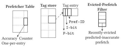
Fig. 3. Implementation of ICP. Thick lines indicate changes introduced by ICP. Each MSHR entry also requires a P-bit. We do not show this in the figure, for clarity.
