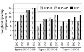
Fig. 8. Effect of varying cache size (percentage on top indicates the peak improvement of ICP for the corresponding category).
