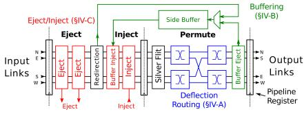
Figure 2. MinBD router pipeline.
