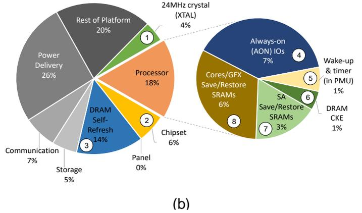
**Figure 1: (a) High level architecture of an Intel Skylake [21] mobile system (processor + chipset). Powered-on system components in DRIPS are highlighted green (numbered) (b) Breakdown of platform power consumption in DRIPS. The total platform power consumption in DRIPS is  $\sim 60$  milli-Watts measured at  $30^\circ\text{C}$  with  $8\text{GB}$  DDR3L-1.6GHz.**
