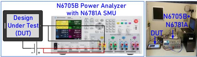
**Figure 5: Platform power measurement infrastructure using a Keysight N6705B power analyzer equipped with a N6781A source measurement unit (SMU).**
