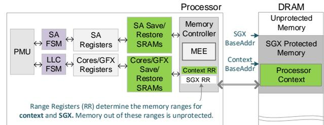
Figure 4: Flow for transferring the processor context into an SGX-protected DRAM area.
