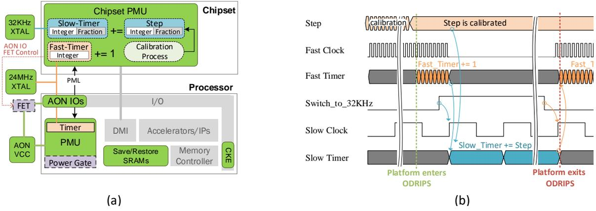
Figure 3: (a) Wake-up event handling and AON IO power-gating. New components are highlighted with dashed lines: Slow-Timer, Fast-Timer, on-board power-gate (i.e., FET) for AON IOs, processor’s PMU power-gate. (b) Timer counting switches from Fast-Timer to Slow-Timer during ODRIPS entry to enable turning off the fast clock crystal oscillator (i.e., 24MHz-XTAL). During ODRIPS exit, timer counting switches back from Slow-Timer to Fast-Timer.
