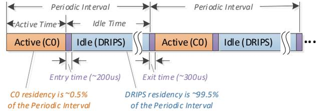
**Figure 2: Average power of an Intel Skylake mobile system in the connected-standby mode, based on our evaluation. 99.5% of the time, the platform is idle (in DRIPS) and consumes tens of milliwatts ( $\sim 60\text{mW}$ ). In the remaining 0.5% of the time, the platform is active (in  $C0$  with display off) and consumes a few watts ( $\sim 3\text{W}$ ).**
