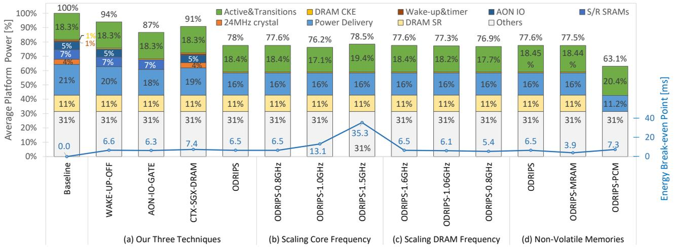
Figure 6: Platform average power consumption and energy break-even point for the baseline and (a) our three power reduction techniques and ODRIPS. (b) ODRIPS while scaling core frequency from 0.8GHz (baseline) to 1GHz and to 1.5GHz, and (c) ODRIPS while scaling DRAM frequency from 1.6GHz (baseline) to 1.06GHz and to 0.8GHz. (d) ODRIPS which uses embedded MRAM (ODRIPS-MRAM) and PCM (ODRIPS-PCM) memory technologies to store the processor context.
