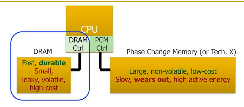
Hardware/software manage data allocation and movement to achieve the best of multiple technologies
