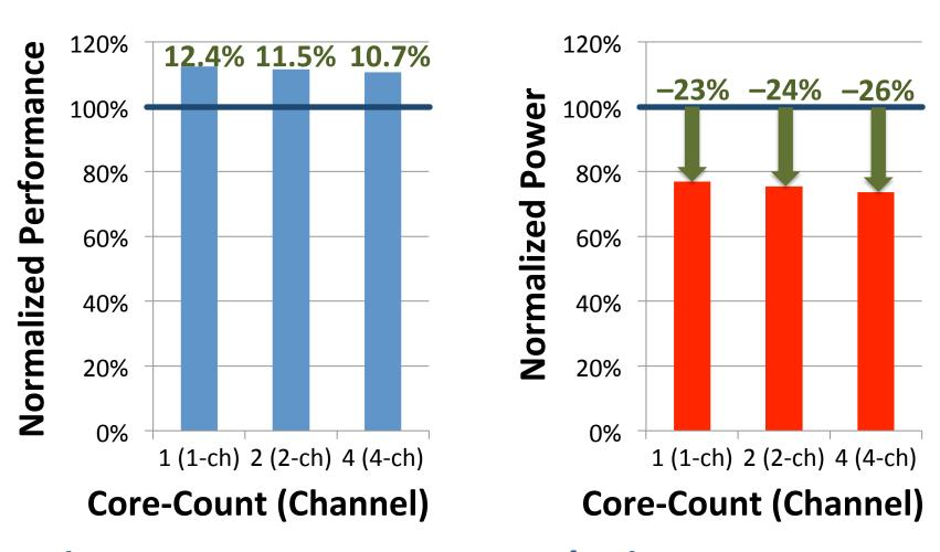
Using near segment as a cache improves performance and reduces power consumption
