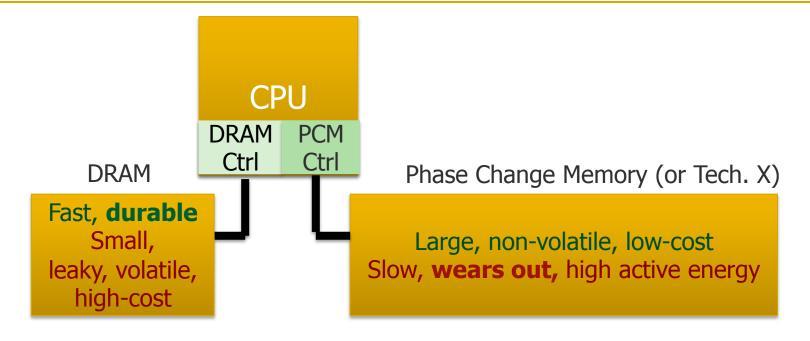
Hardware/software manage data allocation and movement to achieve the best of multiple technologies
