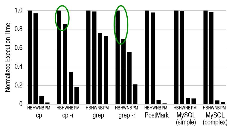
Though, for more complex file system operations like directory traversal (seen with cp -r and grep -r), eliminating the OS/FS overhead improves performance
