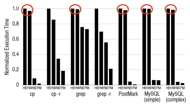
For HDD-based systems, eliminating OS/FS overheads typically leads to small performance improvements → execution time dominated by HDD access latency
