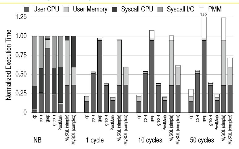
Even if each PMM access takes a non-overlapped 50 cycles (conservative), PMM still provides an overall improvement compared to the NVM baseline
