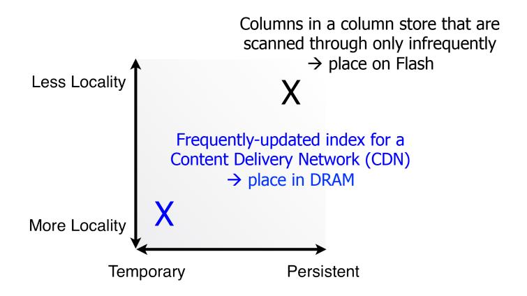
Applications or system software can provide hints for data placement
