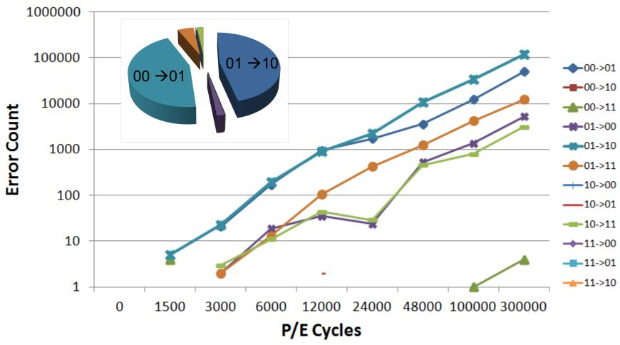
Cells with more programmed electrons tend to suffer more from retention noise (i.e. 00 and 01)
