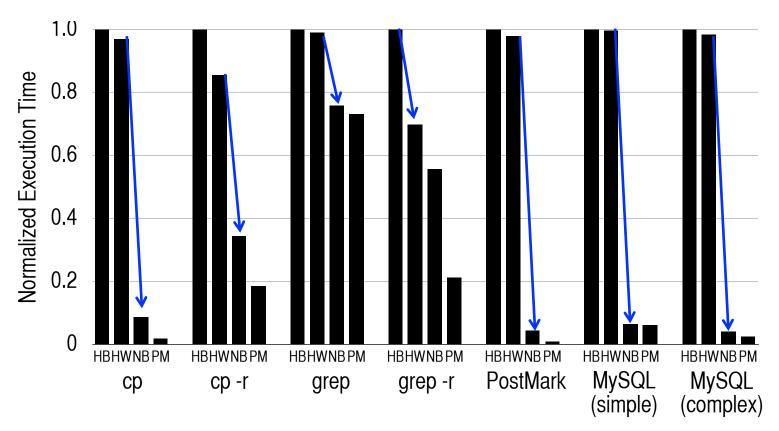
Switching from an HDD to NVM greatly reduces execution time due to NVM's much faster access latencies, especially for I/O-intensive workloads (cp, PostMark, MySQL)
