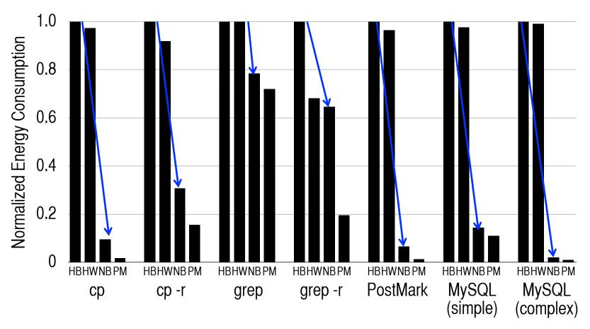
Between HDD-based and NVM-based systems, lower NVM energy leads to greatly reduced energy consumption
