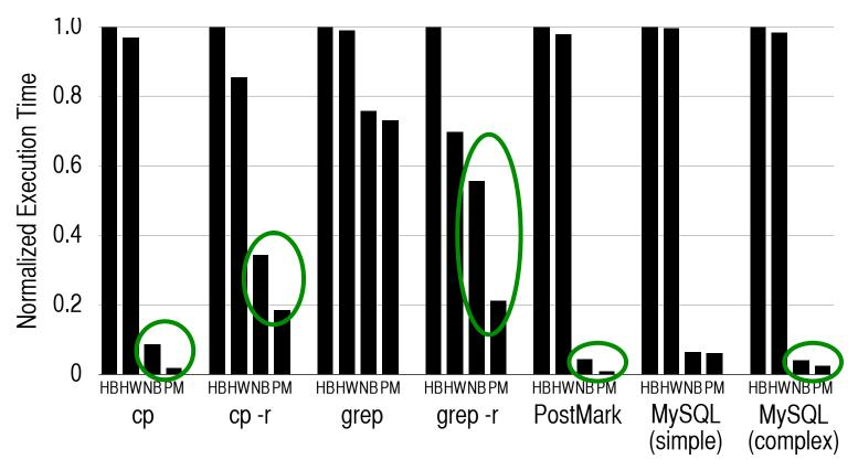
For most workloads, eliminating OS/FS code and buffering improves performance greatly on top of the NVM Baseline system
