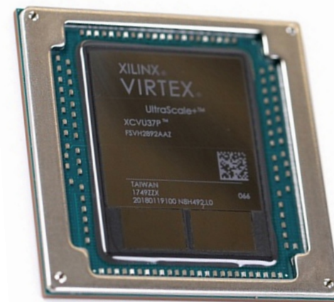
Xilinx FPGA with HBM2 DRAM chips
