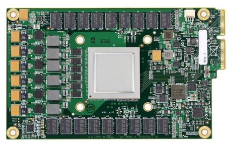
**Figure 3.** TPU Printed Circuit Board. It can be inserted in the slot for an SATA disk in a server, but the card uses PCIe Gen3 x16.
