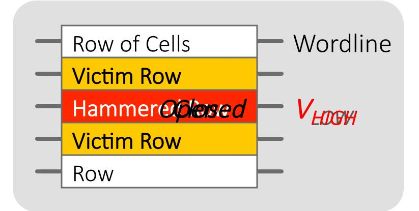
Repeatedly opening and closing a row enough times within a refresh interval induces **disturbance errors** in adjacent rows in **most real DRAM chips you can buy today**
