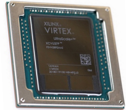
Xilinx FPGA with HBM2 DRAM chips
