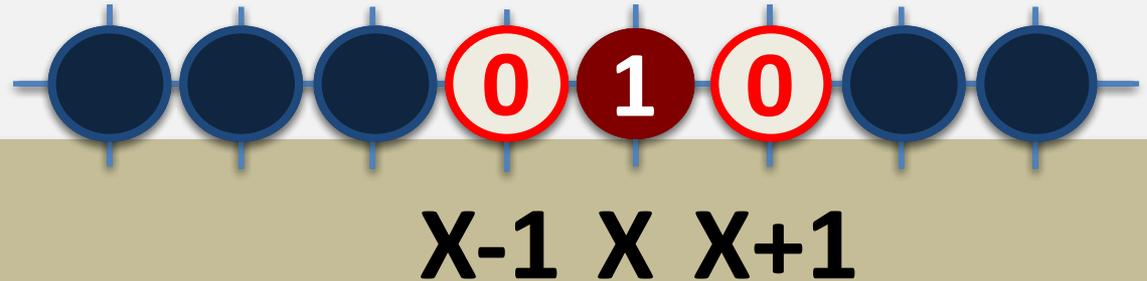
To test cell at ***address  $X$*** , write ***1 at address  $X$***
