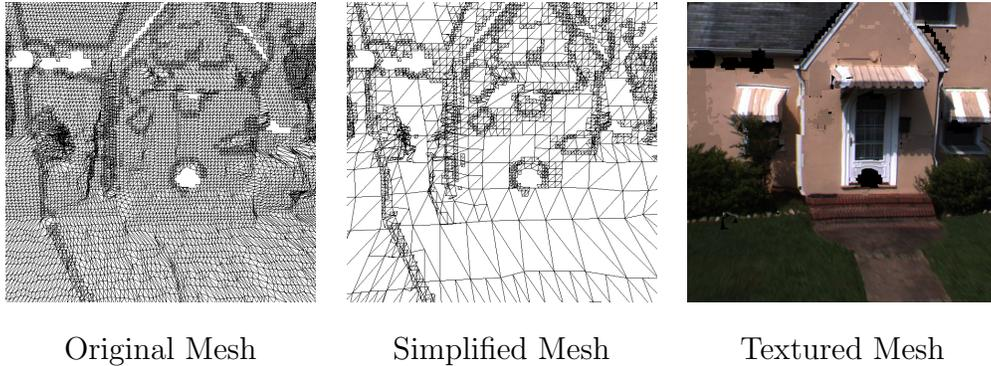
Figure 6: Models are extracted from the fused depthmaps.
