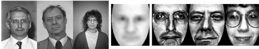
Figure 9.20. Left: Original samples in the FERET database [3]. Middle: The standard mask. Right: The samples after the preprocessing sequence.
