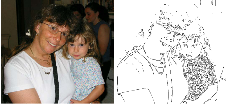
Figure 11.33. Interface Matlab: Left image is the input, right image is after running Canny on it with low/high thresholds 120/200. .
