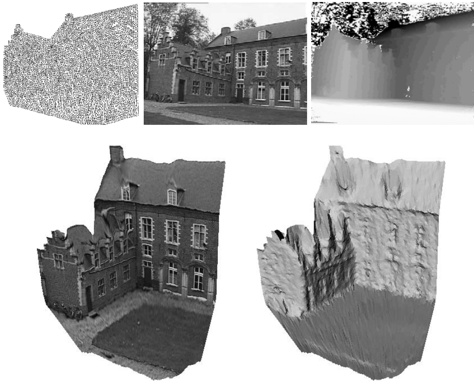
Figure 3.19. Surface reconstruction approach (top): A triangular mesh is overlaid on top of the image. The vertices are back-projected in space according to the depth values. From this a 3D surface model is obtained (bottom)
