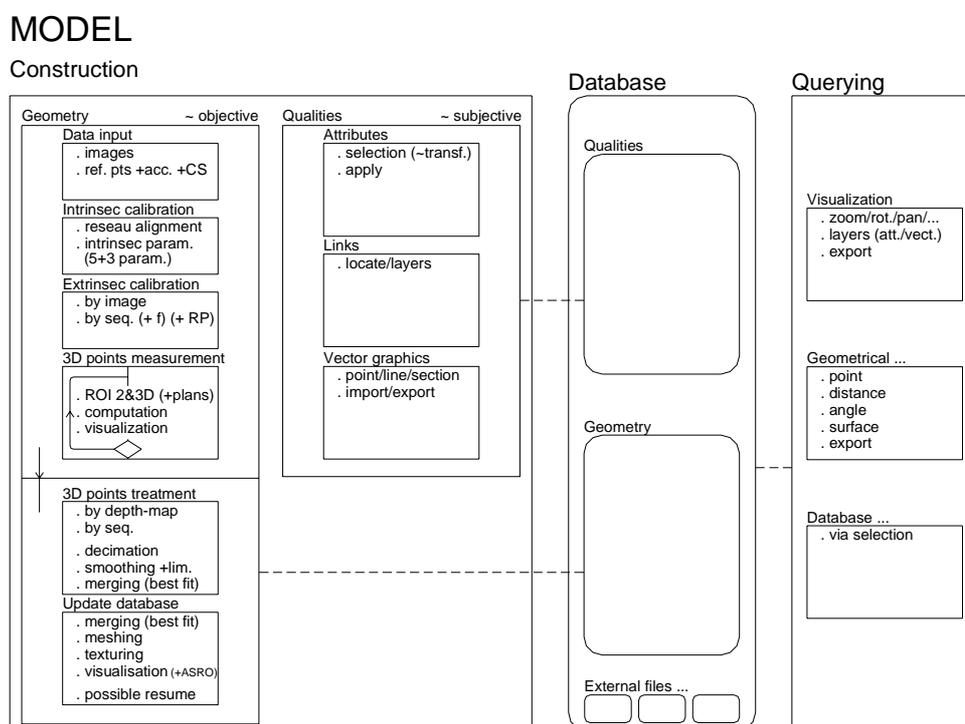
**Figure 2 System structure: model construction - database - database querying**
