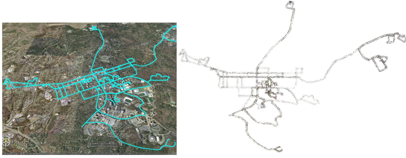
Fig. 9 Map of Chapel Hill, NC, with vehicle path overlaid (left) and top view of recovered reconstruction (right).
