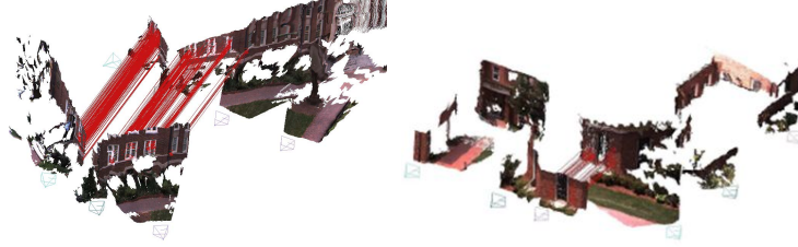
Fig. 14 3D registration of 2 3D models with 45^\circ viewing direction change using VIP features.
