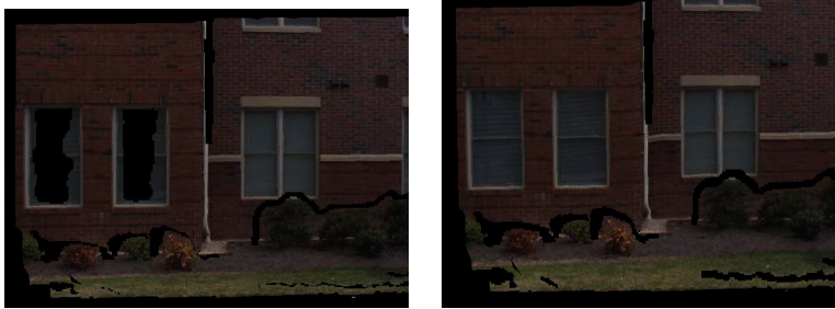
Figure 18: Example of hole-filling. Left: screenshot of original reconstruction. Right: the windows that are not photo-consistent have been filled-in by our algorithm.
