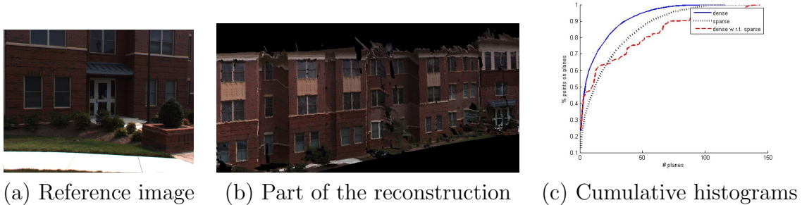
Figure 11: Evaluation of the use of priors. The dotted black curve is the cumulative histogram of the sparse points for the image of (a). The x -axis for the dotted black curve refers to the planes sorted in descending order with respect to the number of points they contain. The solid blue curve is a similar histogram for the dense reconstructed points, with the x -axis in this case corresponding to the planes sorted by the number of dense points they contain. The dashed red curve is a cumulative histogram of the dense points using the ordering of planes according to the sparse points they contain. See the text for more details.
