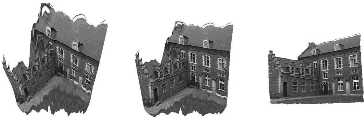
Fig. 9. More perspective views of the 3D reconstruction. Notice that once a 3D reconstruction is available it is easy to generate views which where not present in the original sequence.
