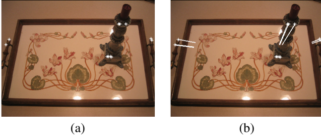
Figure 8. (a) reprojecion error for the projection matrix estimated with QDEGSAC (b) reprojecion error of a RANSAC solution for the projection matrix.
