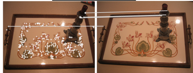
Figure 1. Two views of the tray scene where most matches are on the plane (tray). Only a few matches are on the candlestick (light gray lines). These have to be incorporated to get the correct epipolar geometry.
