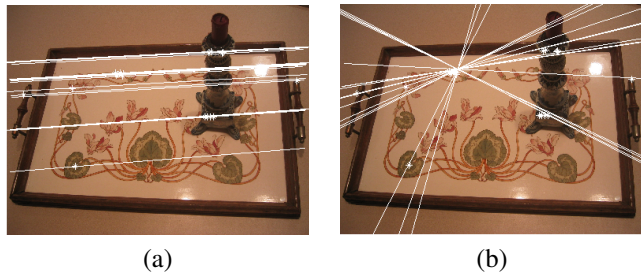
Figure 3. (a) Correct epipolar geometry computed by QDEGSAC valid for all points on the plane and on the candlestick. (b) Epipolar geometry computed by RANSAC only valid for points on the candlestick (plane).
