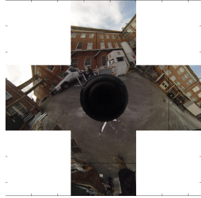
Fig. 13: Cubemap of undistorted left image (unwarping done using a simple line interpolation between angle and r , the distorted radius)
