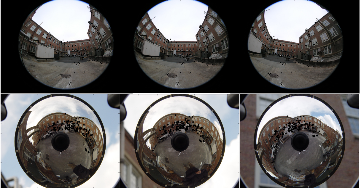
Fig. 9: The triplet of images input to the system with features that were automatically matched overlaid. Top: Fish-eye images Bottom: Catadioptric images
