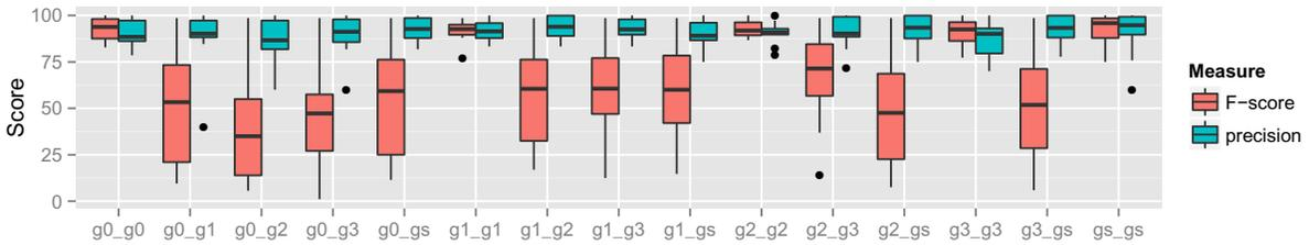
FIGURE 3.12. SLEUTH’s code theft detection performance when the adversary’s compiler is known, so the adversary is using optimization levels to hide his theft; here, we are computing  $Sleuth(5, \langle 1, 60\%, 70\% \rangle, \{gcc\}, \{00, 01, 02, 03, 0s\}, P)$  in Equation 3.6 to generate the sample sets of comparison results that underlie the box plots.
