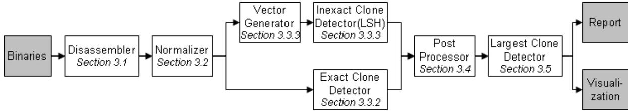
FIGURE 2.1. Disassembly and clone detection process.
