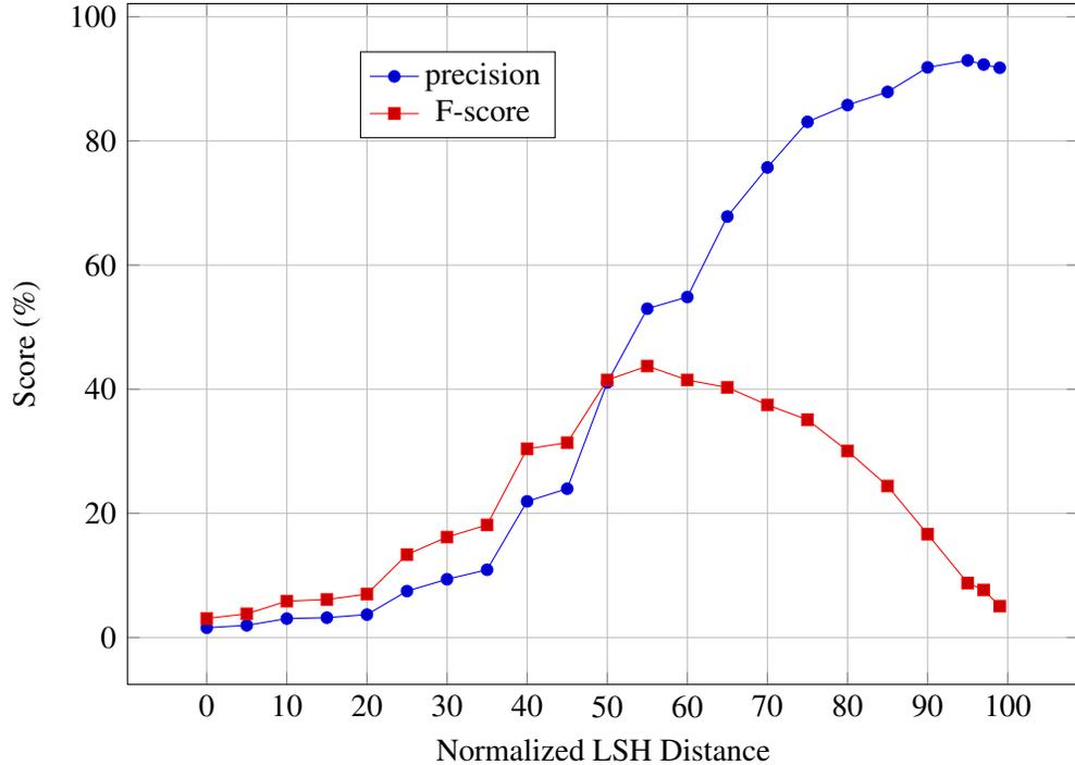
FIGURE 3.5. Effect of minimal allowed output similarity on precision and F-score detecting clones using Sæbjørnsen *et al.* [69] feature vectors.
