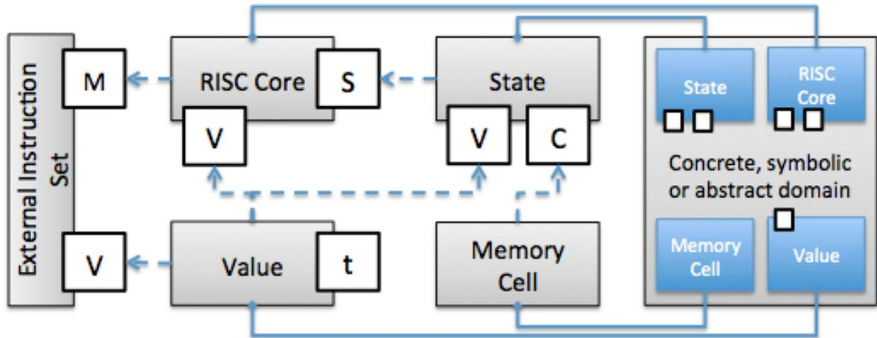
FIGURE 4.6. The architecture of SCOUT.
