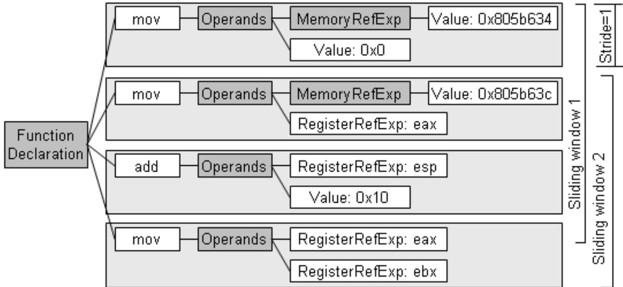
FIGURE 2.2. Example intermediate representation of disassembled binary for stride 1 and window size 3.
