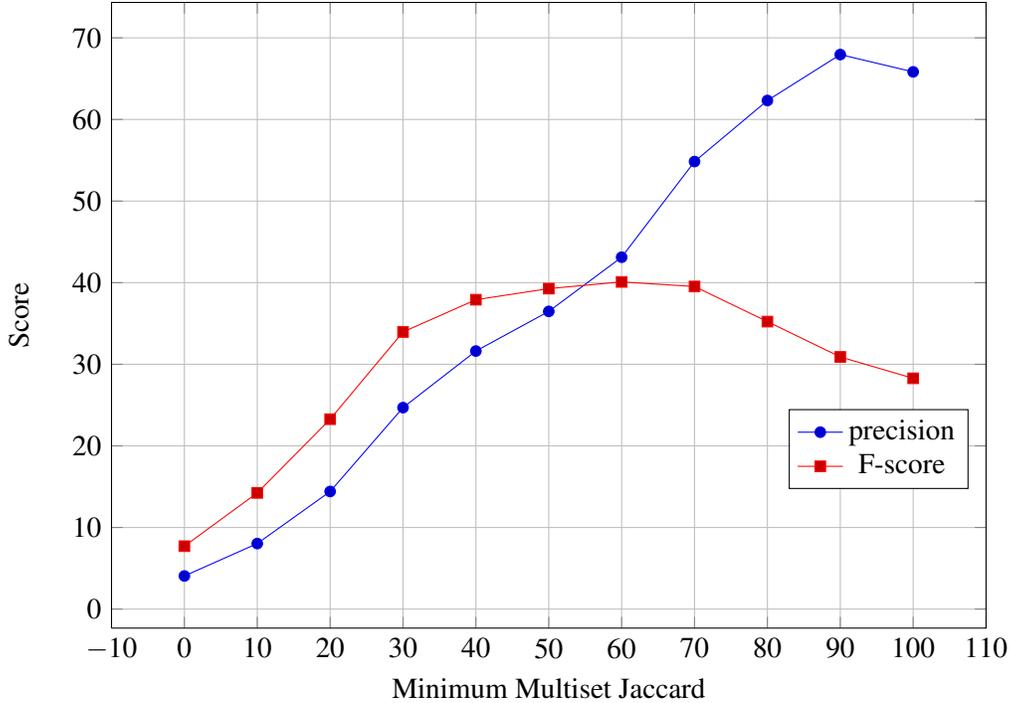
FIGURE 3.9. Static function call measure evaluated with  $Sleuth(5, \langle 1, 0\%, x \rangle, C, X, P)$  where different compilers produce the victim and the suspect ( $c_v \neq c_s$ ) in Equation 3.6.
