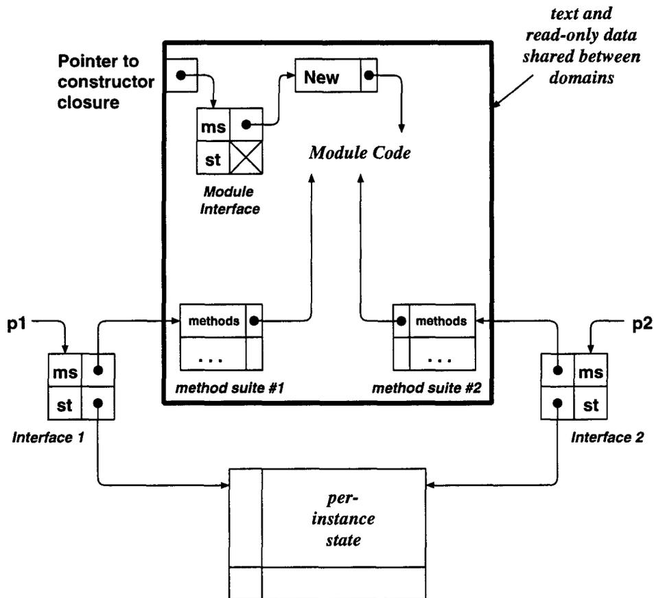
Figure 2: A module implementing an object with two interfaces
