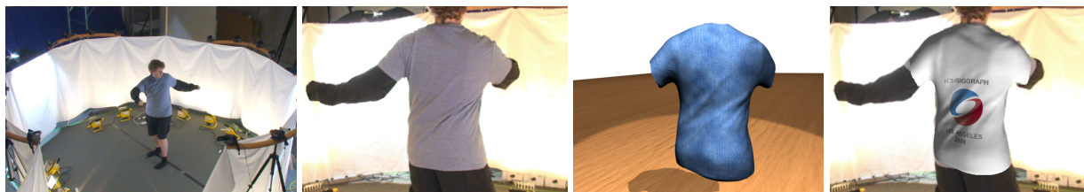
Figure 6.1: Markerless garment capture. From left to right: an actor in the capture setup, one of sixteen viewpoints, the recovered geometry, augmenting the original scene.
