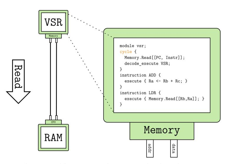
The **cycle** specifies asynchronous behaviour.
