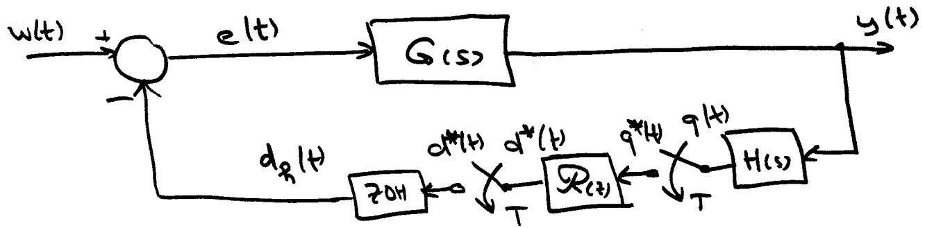
$$\begin{aligned} E(s) &= W(s) - D_H(s) \\ &= W(s) - G_R(s) \cdot D^*(s) \end{aligned}$$
