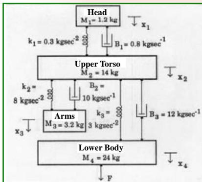
The figure to the left shows a mechanical model of a sitting human body. The legs were left out since they do not contribute to potential oscillations of the upper body. The numerical data are average data for a human adult.
