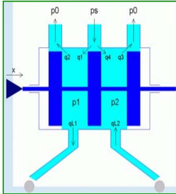
The hydraulic motor is controlled by a servoalve.
