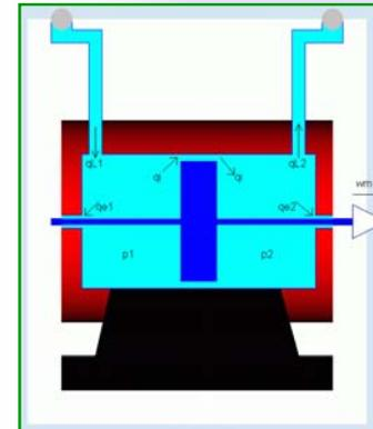
The hydraulic motor has two chambers filled with oil. A wall separates them.
