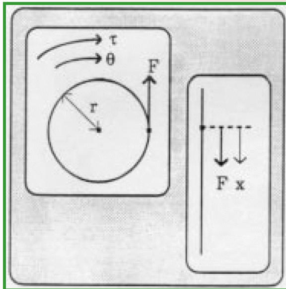
We cut through the gear. The effect of the other body is replaced by a *cutting force*.
