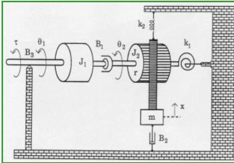
The mixed rotational and translational system exhibits three bodies: the inertiae  $J_1$  and  $J_2$  as well as the mass  $m$ . Therefore, we would expect the system to be of 6<sup>th</sup> order.
