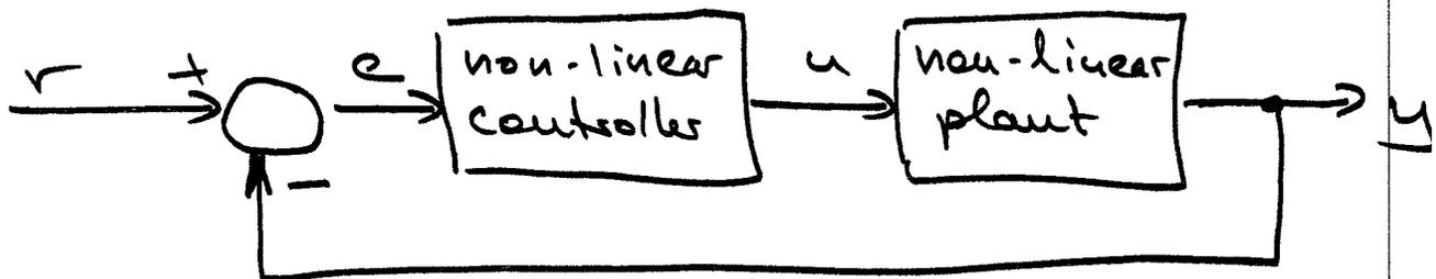
For any given error signal,  $e$ , we need to find the controller output (plant input),  $u$ , that drives the plant output,  $y$ , to where we want it to be; in general, make  $e$  as small as possible.
