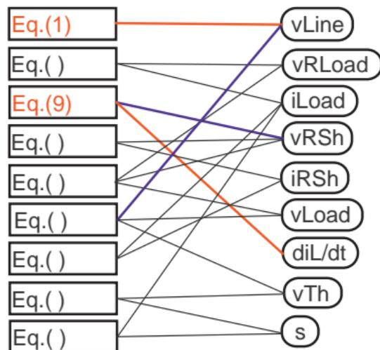
$$1: \quad v_{Line} = V_0 \cdot \sin\left(\frac{2\pi t}{t_p}\right)$$
