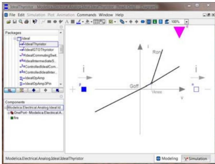
The MSL uses a *leaky diode*.
