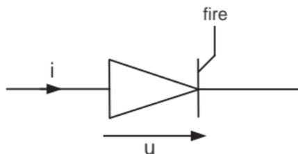
The thyristor is a diode with a modified firing logic. The diode can only close when the external Boolean variable *fire* has a value of *true*. The opening logic is the same as for the regular diode.
