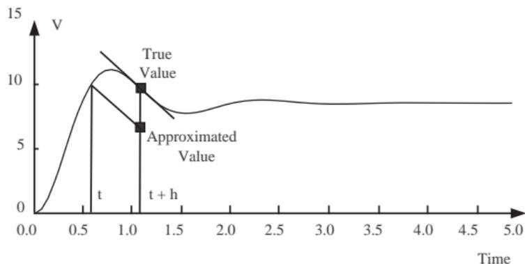
Figure: Numerical integration using the *“BE”* method
