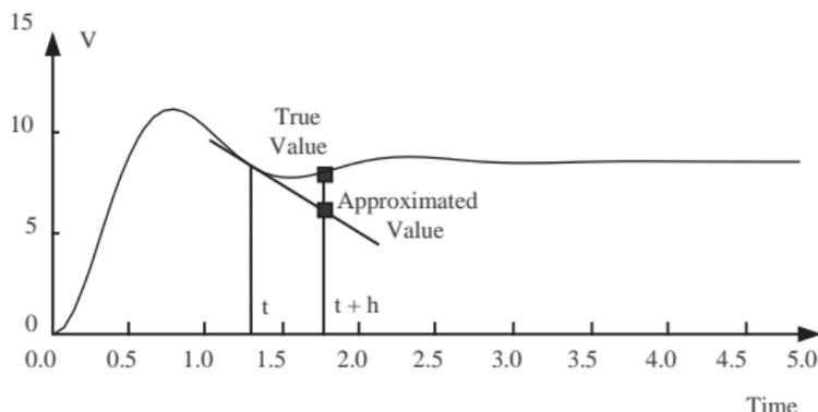
Figure: Numerical integration using the “FE” method
