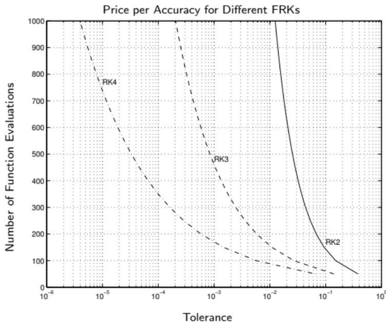
Figure: Simulation efficiency of different FRK algorithms
