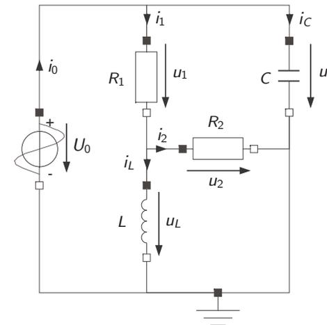
$$\begin{aligned} u_0 &= f(t) \\ u_1 &= R_1 \cdot i_1 \\ u_2 &= R_2 \cdot i_2 \\ u_L &= L \cdot di_L \\ i_C &= C \cdot du_C \\ u_0 &= u_1 + u_L \\ u_C &= u_1 + u_2 \\ u_L &= u_2 \\ i_0 &= i_1 + i_C \\ i_1 &= i_2 + i_L \\ i_L &= \text{pre}(i_L) + h \cdot di_L \\ u_C &= \text{pre}(u_C) + h \cdot du_C \end{aligned}$$
