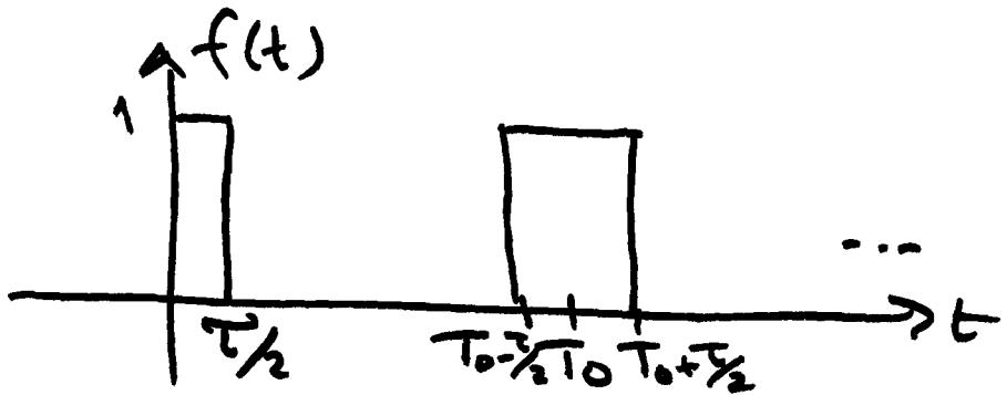
$$P_{av} = \frac{1}{T_0} \int_{T_0/2}^{3T_0/2} |f(t)|^2 dt = \frac{1}{T_0} \left[ \int_0^{T_0/2} 1 dt + \int_{T_0}^{3T_0/2} 1 dt \right]$$
