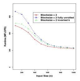
**Fig. 3**. LU blocked algorithm with block size of 2 plotted against several optimizations.
