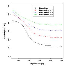
**Fig. 2**. LU Baseline algorithm plotted against the Blocked algorithm with varying block sizes.
