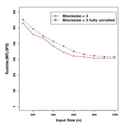
**Fig. 4**. LU blocked algorithm with block size of 3 plotted against a loop unrolled implementation.
