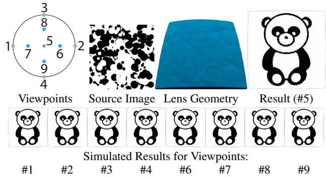
**Figure 14:** We induce a stable viewing zone by exploiting multi-view lens generation in a novel way: by using the *same* target images at each of the nine views, arranged in the layout on the left. The lens consists of  $128 \times 128$  facets.
