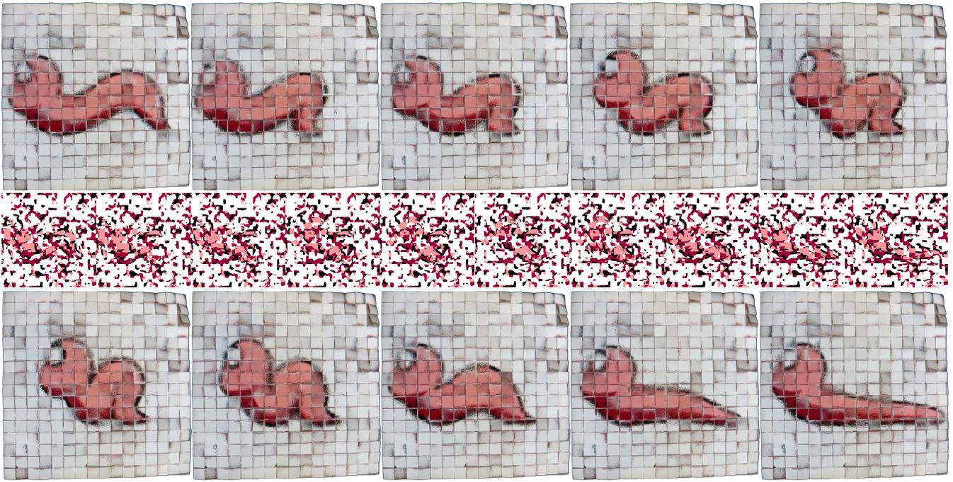
**Figure 9:** Warping an unstructured video sequence with a universal lens with  $16 \times 16$  facets. The middle row has the different (shrunk) source images, and the top and bottom rows are photographs of a manufactured lens placed over the source images as they animate.
