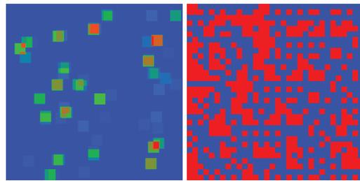
**Figure 7:** Heatmap for a source-optimized lens (left) with values from 0 (blue) to 18 (red) overlaps. Clearly, several facets are matched to the same source patch. The heatmap for a universal lens (right) illustrates the injective mapping: red corresponds to a single match and blue to no match.
