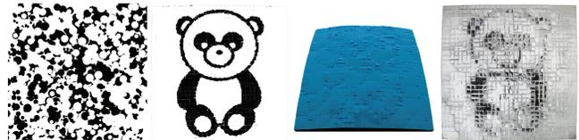
**Figure 11:** A physically milled result. Simulation (middle left) closely matches the target, however the smooth lens (middle right;  $32 \times 32$  facets with  $11 \times 11$  micro-facets) is degraded during milling and manual polishing, resulting in a lower quality physical result (right) than that of a 3D printer (see Figure 12).
