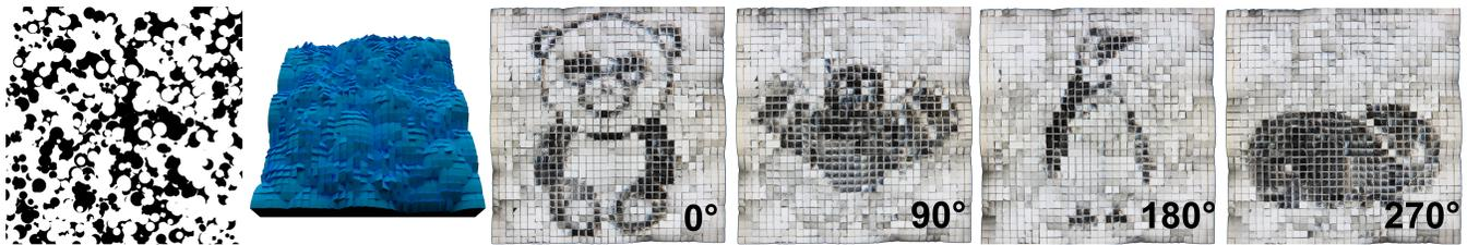
**Figure 1:** We automatically design and manufacture magic lenses to warp source images into specified target images. Here we photograph a source image (far left) viewed through a manufactured lens with  $32 \times 32$  facets (left), resulting in four images depending on the lens' orientation atop the source.
