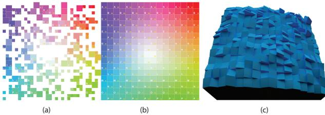
**Figure 15:** Visualization of the warping behavior of a universal lens with  $16 \times 16$  facets: Given the target image (b) and lens geometry (c), we compute the source image (a) using our inpainting method.
